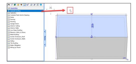
For a natively drawn Roofplan, to apply an Assembly to a specific roof facet: highlight the facet by clicking on it, and then drag-and-drop the Assembly icon directly onto the facet.
